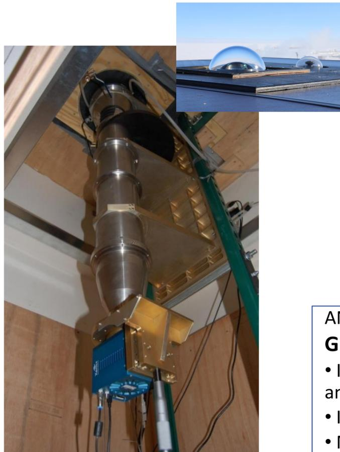
Figure 2: Advanced Mesospheric Temperature Mapper (AMTM) imager at the South Pole station
