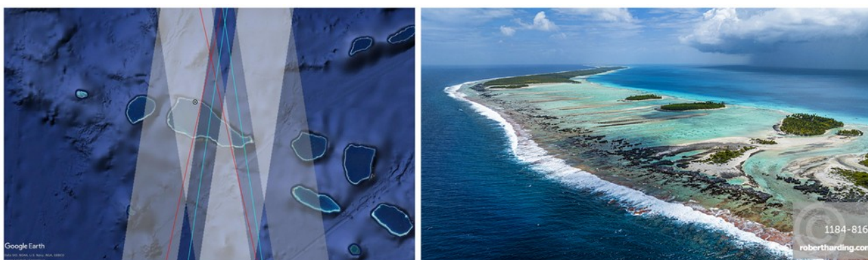
(Left) Google Earth map of Rangiroa atoll, at the western edge of the Tuamotu archipelago, with Sentinel-3A tracks (red lines) and SWOT nadir tracks (blue lines) and left/right swath (shaded area); (Right) Aerial photograph of a section of the southern barrier reef of Rangiroa atoll showing wave breaking over the reef top (credit: Robert Harding)
